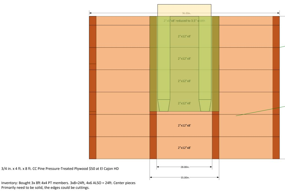
PT Plywood- do I have a 48" x 35" piece? Or multiple strips of 35" lengths? This piece is intended to prevent tip-overs when picked up by forklift. Forkliftable Base of 4x4 PT timbers, subfloor of 2" PT wood, 2x12 shown. Use 2x4 "stud" spaces in floor for an insulation cavity. Top with OSB ¾" sheet. For forklift anti-tipping safety, some 1x4 PT strips across bottom edge of 4x4's, or strips from ¾ pt plywood. Do I have some remnants?
